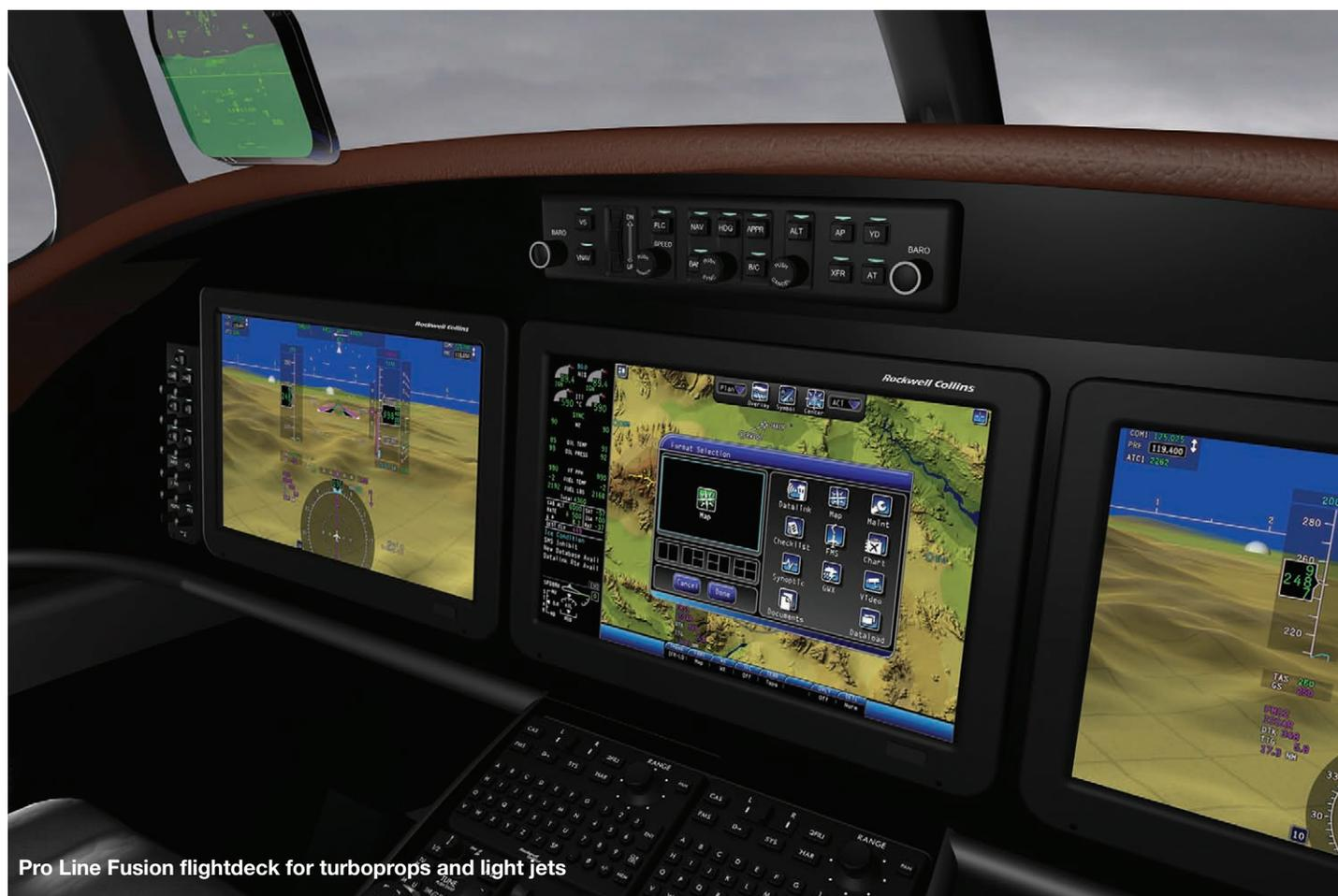
Pro Line Fusion flightdeck for turboprops and light jets
